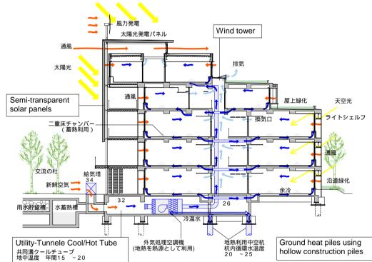
Fig2, Cross-section of the Lecture-Hall & Laboratory Building, showing the natural energy flow system
